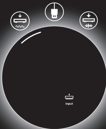
Touch the mu-so input icon to select the analogue, USB and digital inputs sequentially.
