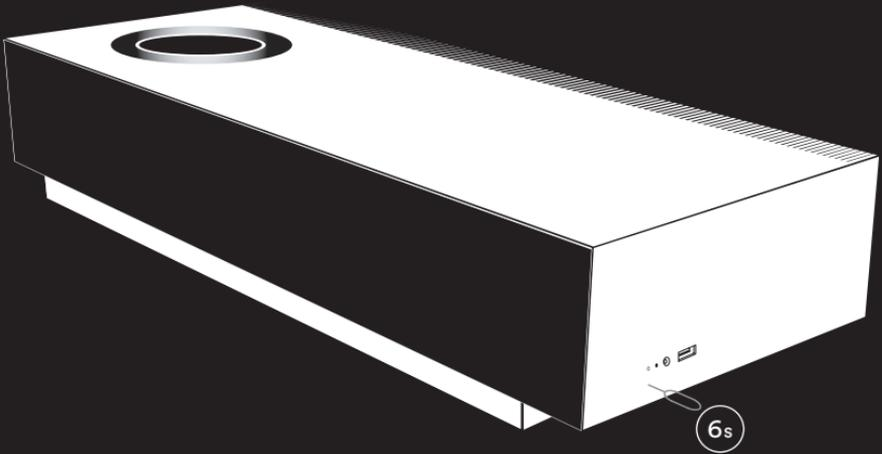
Press and hold the pin-hole button for six seconds to reset mu-so defaults.
