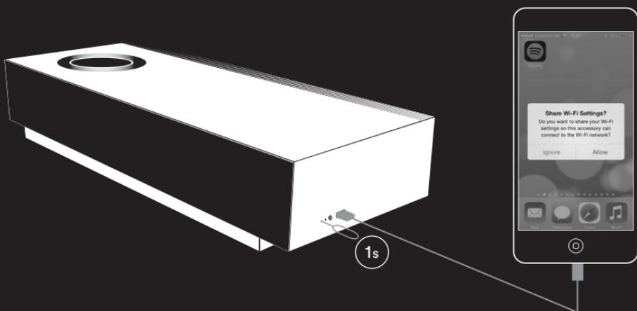
Connect iOS (> v6.0) device. Press and release mu-so pin-hole button.
