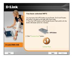
Press the WPS button on your access point or wireless router within 2 minutes to establish connectivity.
