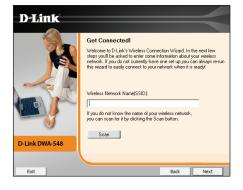
Click the **Scan** button to display a list of wireless networks (site survey). Click on the network name (SSID) and click **Next**.
