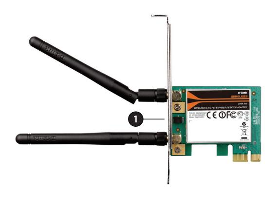
1 WLAN LED The LED will blink when the wireless adapter is operating correctly.
