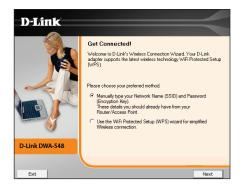
Enter the network name (SSID) manually. If you enter the SSID incorrectly, you will automatically be brought to the site survey page. Click **Scan** to display the site survey page. Click **Next** to continue.
